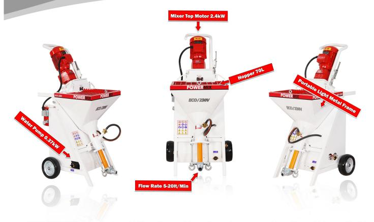
POWERMIX ECO is a single phase 230V, continues mixing and spraying pump machine with very high capacity. It is suitable for plastering premixed gypsum, lime and cement based plasters, glues, colored plasters, stuccoes and finishing coats. It is perfect option for construction works in residential areas due to it can be operated with 230V residential electricity.
